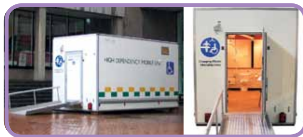
Birmingham city centre provided a Changing Places toilet for visitors to their Christmas market and busy shopping district, supplied by Andy Loos. A straight-on, ramped approach provides easy access
